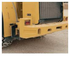
**Counterweight.** The one-piece counterweight is integrated into the 962H design and styling. This 3084 lb (1399 kg) counterweight incorporates the rear lights into the top of the structure.
