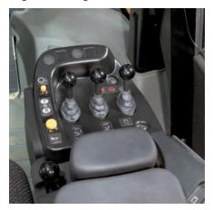
**Seat.** The Cat C-500 Series Comfort air suspension seat, standard in the 962H, is built strong and durable and is 6-way adjustable to accommodate all-sized operators. The cast one-piece back and seat pan prevent protrusions under the cushions. The seat features an automotive-style lumbar support for maximum comfort. The right hand armrest with integrated implement controls adjusts for comfortable, convenient operation. A heated seat option is available for additional comfort.
