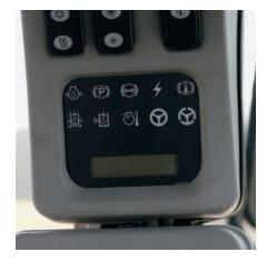
Caterpillar Monitoring System. The 962H is equipped with the Cat Monitoring System (CMS) that keeps watch over the health of your loader. CMS monitors critical engine system functions and will derate the engine to protect itself from damage if needed. Depending on which of the following six critical conditions arise, the CMS monitor or front panel will display warning lights and sound audible alarms.
