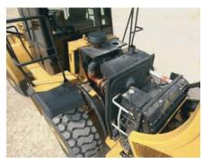
**ENGINE COMPARTMENT ACCESS.** The non-metallic hood on the 962H has been redesigned and restyled from previous models. Side and top panels are stronger due to more robust reinforcement ribs - the change in contour also adds to rigidity of the hood.
