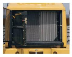
**COOLING SYSTEM.** Cooling system access for clean-out and maintenance is outstanding. The perforated and corrugated grill minimizes debris build-up and swings out for easy cleaning and access to the cooling cores.
