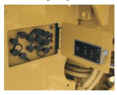
**REMOTE PRESSURE TAPS.** Pressure taps for the steering and hydraulic systems, transmission (optional) and brakes are grouped behind an access panel just below the right-side service platform.
